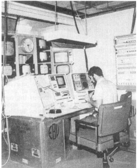
The EBU's mobile master control equipment was used in Montreal for the first time.
